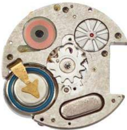
7P, at the time the thinnest quartz movement in the world, 1976
